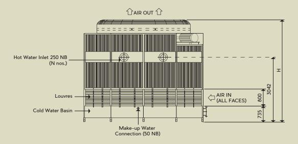
TYPICAL TOWER SCHEMATICS - PLAN VIEW AND ELEVATION (SINGLE CELL) FOR DETAILED ENGINEERING DATA SEE TABLE 1 ON NEXT PAGE
