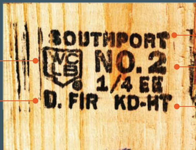
WEST COAST LUMBER INSPECTION BUREAU'S STRENGTH GRADING STAMP
