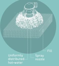
Nozzles are designed to uniformly distribute water over maximum area
