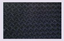
**ELIMINATOR:** Drift eliminator panels are formed from 0.5 mm thick PVC sheets into a cellular configuration which forces exhaust air into three complete directional changes to eliminate water droplets from the air stream. The 3-pass eliminator provides maximum efficiency in elimination up to 0.005% of circulating water flowrate at the very minimum in horse power consumption. These also have a flame spread rating less than 25 mm as per ASTM D635.
